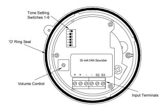
Fig 2 Location of field terminals and controls.
