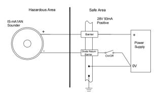
Fig 5 Single stage alarm using two channel barrier.
