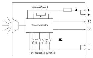
Fig 1 Simplified block diagram
