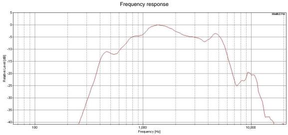
Note: The frequency response is derived using a Swept sine method.
