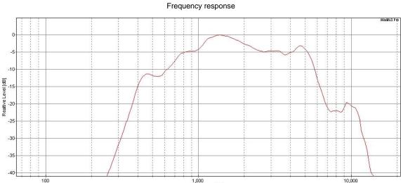
Note: The frequency response is derived using a Swept sine method.
