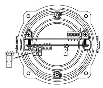
J2 Header Pin - <u>Postion A</u>, Factory default position (pins 1 & 2 linked) removes power supply TB Fault resistor & RLY 1-2 out of circuit.
