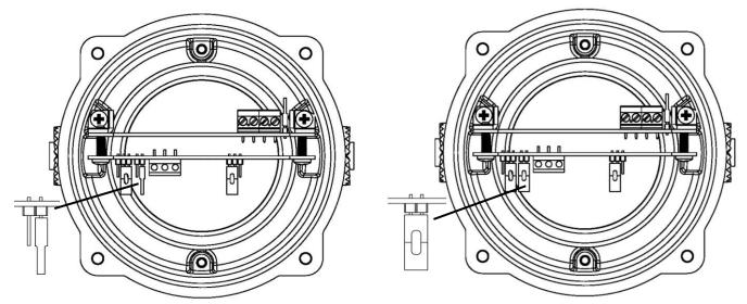
J1 Header Pin - <u>Postion A</u>, Factory default position (pins 1 & 2 not linked) places TB1 Current sense resistor in circuit.
