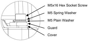
Fig. 13 Cover and Guard Fixtures
