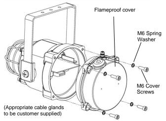
Fig. 2 Accessing the Explosion proof Enclosure.
