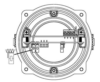
J2 Header Pin - <u>Postion B</u> (pins 2 & 3 linked) places power supply TB Fault resistor & RLY 1-2
