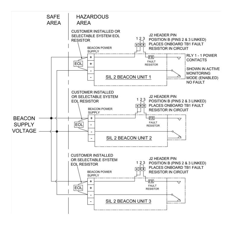
Figure 17: Schematic of SIL 2 system wiring for fault detection in standby mode only – 2 wire installation configuration in star formation
