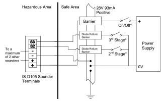
Fig 6 Multi stage alarm using Zener barriers.
