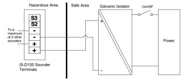
Fig 7 Single stage alarm using galvanic isolator.
