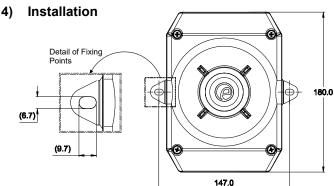
Fig 3 Fixing hole locations
