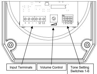
Fig 2 Location of field terminals and controls.
