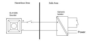
Fig 6 Single stage alarm using galvanic isolator.
