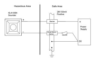
Fig 4 Single stage alarm using two channel barrier.
