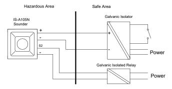
Fig 7 Multi stage alarm using galvanic isolated relays
