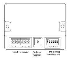
Fig 2 Location of field terminals and controls.
