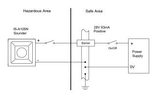
Fig 3 Single stage alarm using single channel barrier.
