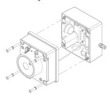
Once the screws are removed the cover will hand down out of the way to gain access to the Ex e terminal block, the internal earth terminal and mounting hole recesses.
