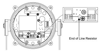
Fig. 9b End of Line Resistor Placement
