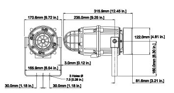
Fig. 1b Fixing Location for Combined Sounder Beacon Radial
