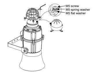
Fig. 12 Replacement of beacon lens cover
