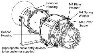
Fig. 2 Accessing the Enclosure.
