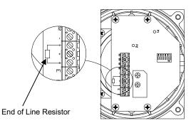
Fig. 8 End of Line Resistor Placement
