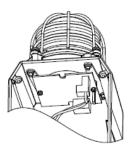
The xenon beacon is set as standard to 1Hz flash rate mode but it can be set to either 1.5Hz flash rate or double Strike flash pattern modes also. To alter the settings, change the position of the header pin as shown:
