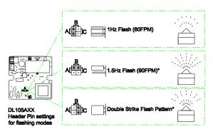
The LED beacon is set as standard to the 2Hz flash mode but it can be set to a steady on mode also. To alter the settings, change the position of the header pin as shown.
