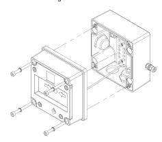
Once the screws are removed the cover will hang down out of the way to gain access to the terminal block, the internal earth terminal and mounting hole recesses.
