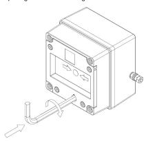
The test key is inserted in the test cam and rotated clockwise by an angle of 60° the glass element will visibly drop down in the viewable window.
