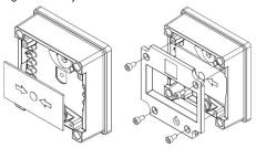
To fit the new glass element rotate the top cam clockwise by an angle of 50° (use a 6mm Allen key) this will than allow the glass to fit back into the pocket it sits in, resting on the pivot point and test cam, release the top cam to rest on the top of the glass element.
