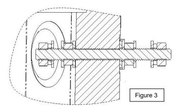
When using the external earth terminal a cable crimp lug must be used. The cable lug should be located between the two M4 stainless steel flat washers. The M4 stainless steel spring washer must be fixed between the outer flat washer and the M4 stainless steel nut to ensure that the cable lug is secured against loosening and twisting.
