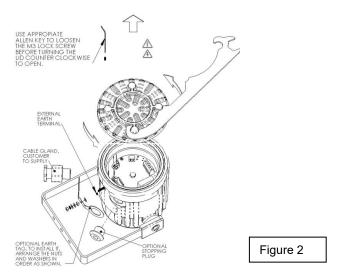
On completion of the cable wiring installation the flameproof joints should be inspected to ensure that they are clean and that they have not been damaged during installation. Also check that the 'O' ring seal is in place. When replacing the flameproof cover ensure that it is tighten fully with tool provided.
