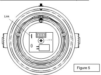
GNExL2 and GNExL1 8 ohm and 16 ohm low impedance loudspeakers have dual input terminals on the pcb assembly for input and output wiring. A cable of up to 2.5mm² can be connected to each terminal. If dc line monitoring is used cut the link on the board (see figure 5 and section 14 of this manual).
