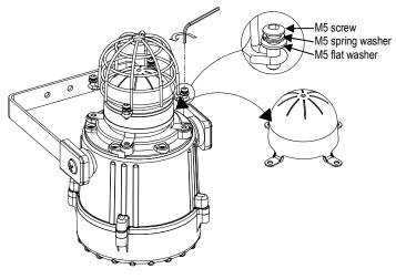
Fig. 11 Replacement of beacon lens cover
