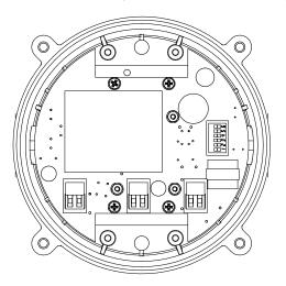
Fig. 9: DIP Switch Location
