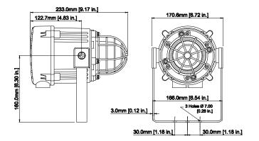
Fig. 1 Fixing Location for Beacon
