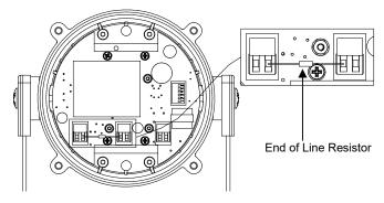
Fig. 8b End of Line Resistor Placement
