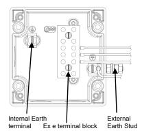
Note: Depending on options chosen an 8-Way DIN Rail or 6-Way terminal block may be selected.
