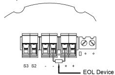
Figure 9: End of Line Resistor placement.
