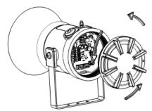
Fig 2: Accessing the enclosure
