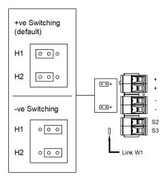
Figure 7: Stage Switching Polarity.
